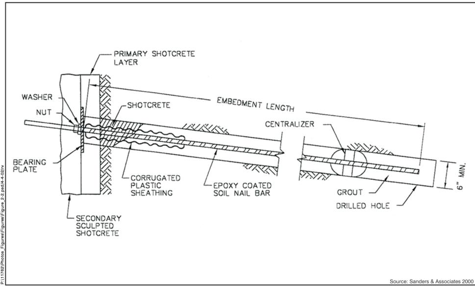
Soil nails are structural high-strength rebars, grouted into drilled holes and inclined slightly downward into the soil.
